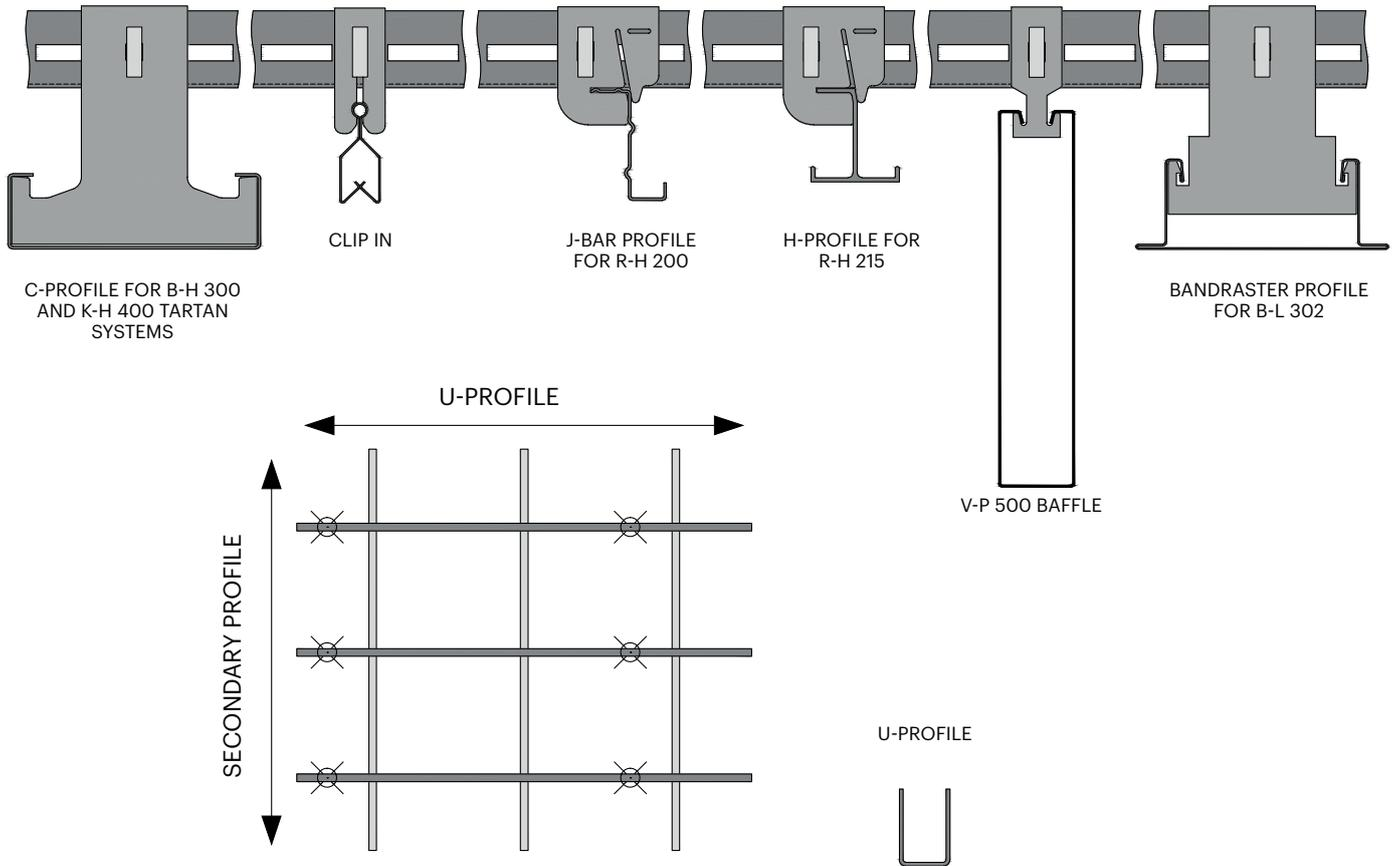
U-PROFILE TYPICALLY INSTALLED AT 1200MM CENTRES AND SUSPENDED AT 1200MM ALONG LENGTH. REFER TO INSTALLATION GUIDE FOR DETAILS.
