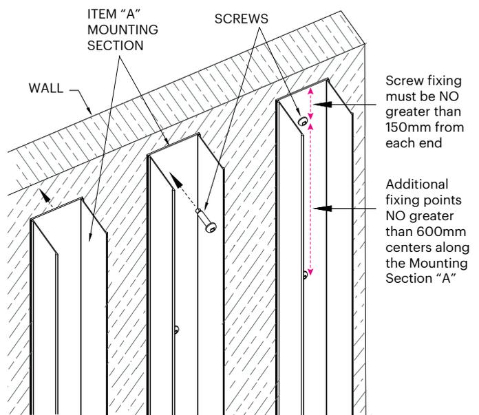
3. The Baffle Mounting Section is to be screw fixed to the substrate. The screw fixing must be no greater than 150mm from each end, with additional fixing points no greater than 600 mm centers along the Mounting Section.
