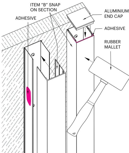
6. End caps can be supplied for all Snap On Baffle profiles and are friction fitted. When installing End Caps, apply a "thumb print sized" dab of construction adhesive to ensure suitable fitting.
