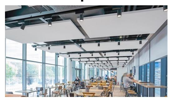
Rockfon Eclipse Panels can be suspended from almost any substrate, and give the appearance of effortlessly floating in any room. An almost unlimited colour range is available to designers as well as a large range of shapes and custom sizes. They are quick to install and have a high dimensional stability for demanding environments.
