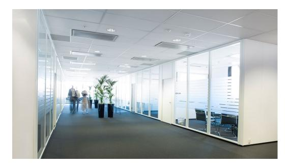
Rockfon Sonar dB 35 has excellent light reflection properties and painted edges for durability in corporate offices or facilities that require frequent access to the ceiling plenum. With high-performance acoustics up to NRC 0.85, Rockfon Sonar dB 35 has the additional benefit of room-to-room sound attenuation control when plenum barriers are impractical and where disturbance control is required.
