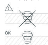
Pig Tail Hook Installation
